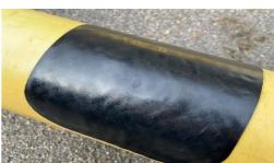
**Kebulen Patch C 50** consists of a stabilized and cross-linked polyethylene carrier film coated on one side with a thermoplastic hotmelt adhesive. The outer side of the patch is embossed with a tactile thermal indicator, so that during processing it is possible to recognize when the processing temperature has been reached by the smoothing process. It's compatible with factory coatings made of PE, PP, FBE, PU and Bitumen.
